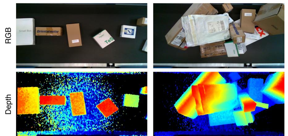
Data from the Intel Realsense Lidar RGB-D camera.
