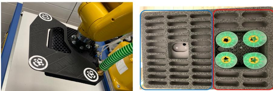
The 3D-printed vacuum gripper developed uses a combination of foam and suction cups with multiple gripping zones. Camera-robot calibration is achieved with an adapter plate with CCTags on the gripper.
