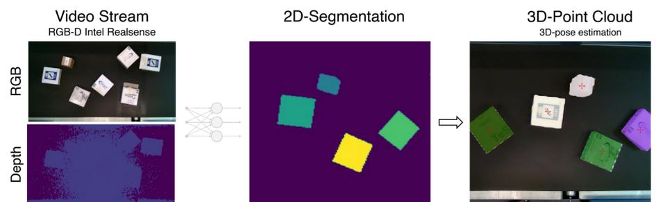
Overview of the image processing. First the parcels are segmented by a neuronal network. Then the 3D pose is estimated and sent to the robot.
